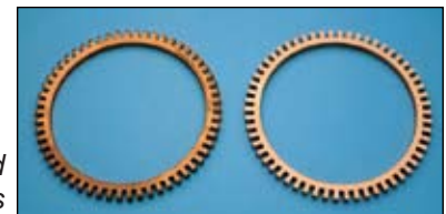
Collar deburred with glass beads
