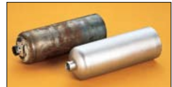
Cylinder surface profiled with ALOX
